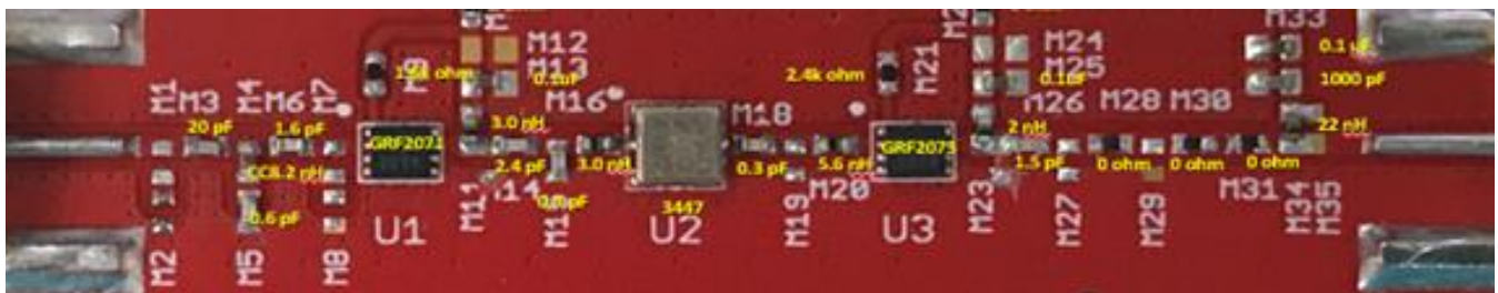
Figure 2. Guerrilla RF’s Single SAW SDARS Reference Design
