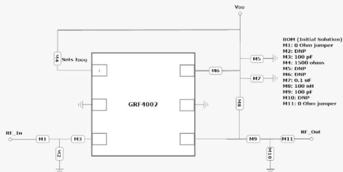
For the given initial requirements, [GRF4002](#) has proven to be an excellent solution. But let's say the system dynamic range requirements change and it is determined that your LNA must offer a low-loss bypass capability which GRF4002 does not provide; the other RF requirements remain unchanged. Luckily, thanks to the breadth of the Guerrilla RF DFN-6 portfolio, a drop-in solution to the new requirement exists and it is called [GRF4142](#).
