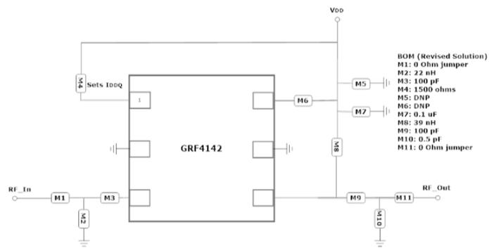
The example above showed how a completely new performance capability (bypass) could be accommodated by a single layout using the Guerrilla RF DFN-6 layout and general purpose schematic. The need to revise the layout for a new part/package was avoided.
