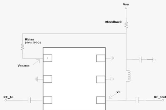
Often the problem is solved by selecting a device with the desired  $P_{sat}$  characteristic. When such a device can't be found, there is a simple, but effective, way to limit  $P_{sat}$  by using resistive feedback. The feedback resistor is placed in series with the driver amplifier power supply. Note that this effort to limit driver  $P_{sat}$  assumes that linearity is not a concern.
